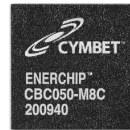
8 mm x 8 mm QFN SMT Package
